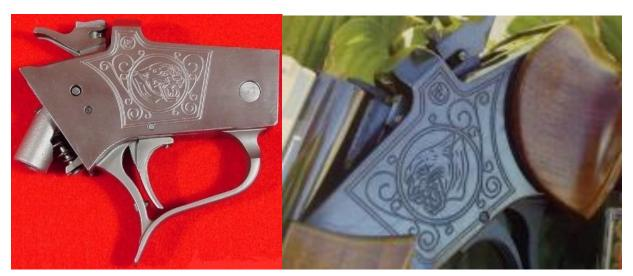
At this time T/C's custom shop Fox Ridge also offered flat-side frames in both blued and stainless steel. Note the pivot pin location of the easy open style being placed just above the trigger (the trigger which is a change too when the easy open frames came out) and the selector style hammer on this stainless custom shop flat-side. I also attached the IHMSA flat-side here too so you can easily see the difference in the two.
