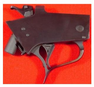
It is important to point out as an upgrade to the older Contender frames you could send them in and be converted to the "Easy Open" design. By doing so they drilled the pivot pin location and put the next version of the hammer on them with the selector safety along with the newer trigger group.
